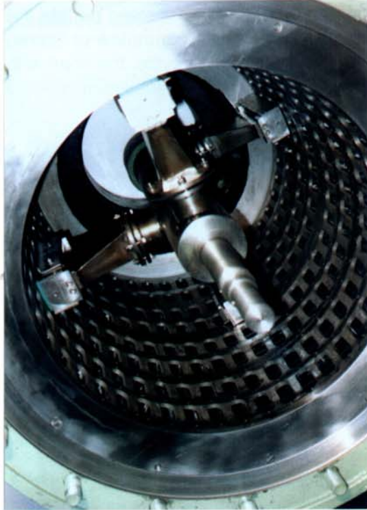
Detail of a filtration cage of a chamber screen and suction pipes of FILTROMAX TMF
